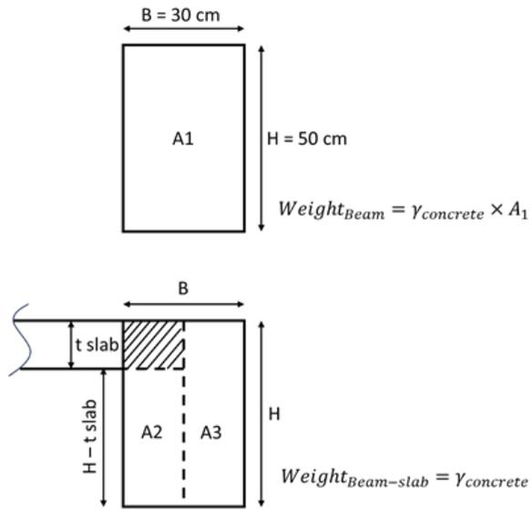
$$\frac{Weight_{Beam-slab}}{Weight_{Beam}} = \frac{\gamma_{concrete} \times (A_2 \times A_3)}{\gamma_{concrete} \times A_1}$$
